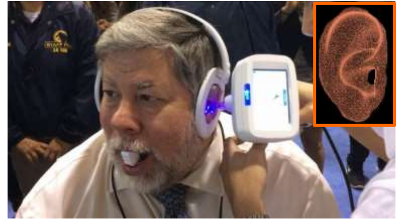
High Resolution Ear Scanner for audiologists (>10k€)
